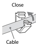
Rotate to unlock the HDMI cable holder first, then remove it.
