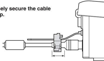
Loosely secure the cable clamp in the area shown above.
