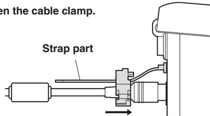
Take hold of the strap part, slide the cable clamp until it stops moving, and then secure it tightly.
