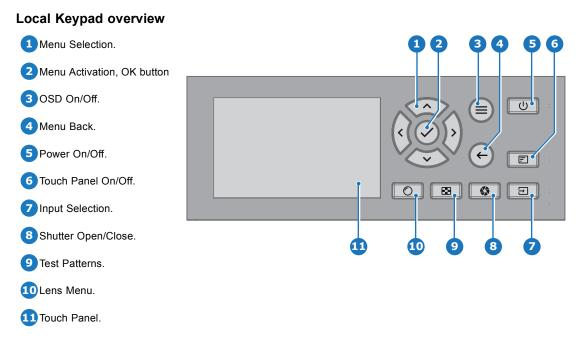
The Keypad gives direct access to several functions, in addition to access to the menu system.
