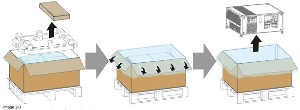
Remove accessory box, polymeric foam and projector
