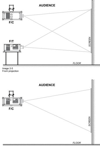
Image 2-6 Front projection, Ceiling mounted, in table position
