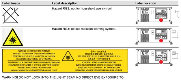
THE BEAM IS PERMITTED. RG3 IEC EN 62471–5:2015. CLASS 1 IEC EN 60825–1:2014. HAZARD DISTANCE: CONSULT SAFETY MANUAL.
